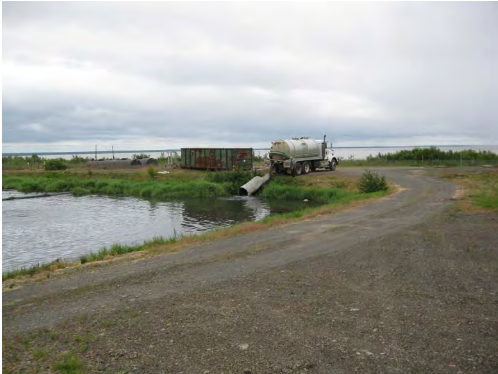
Photo 14 - Pumper Truck Dumping into Southeast Corner of Cell #1
