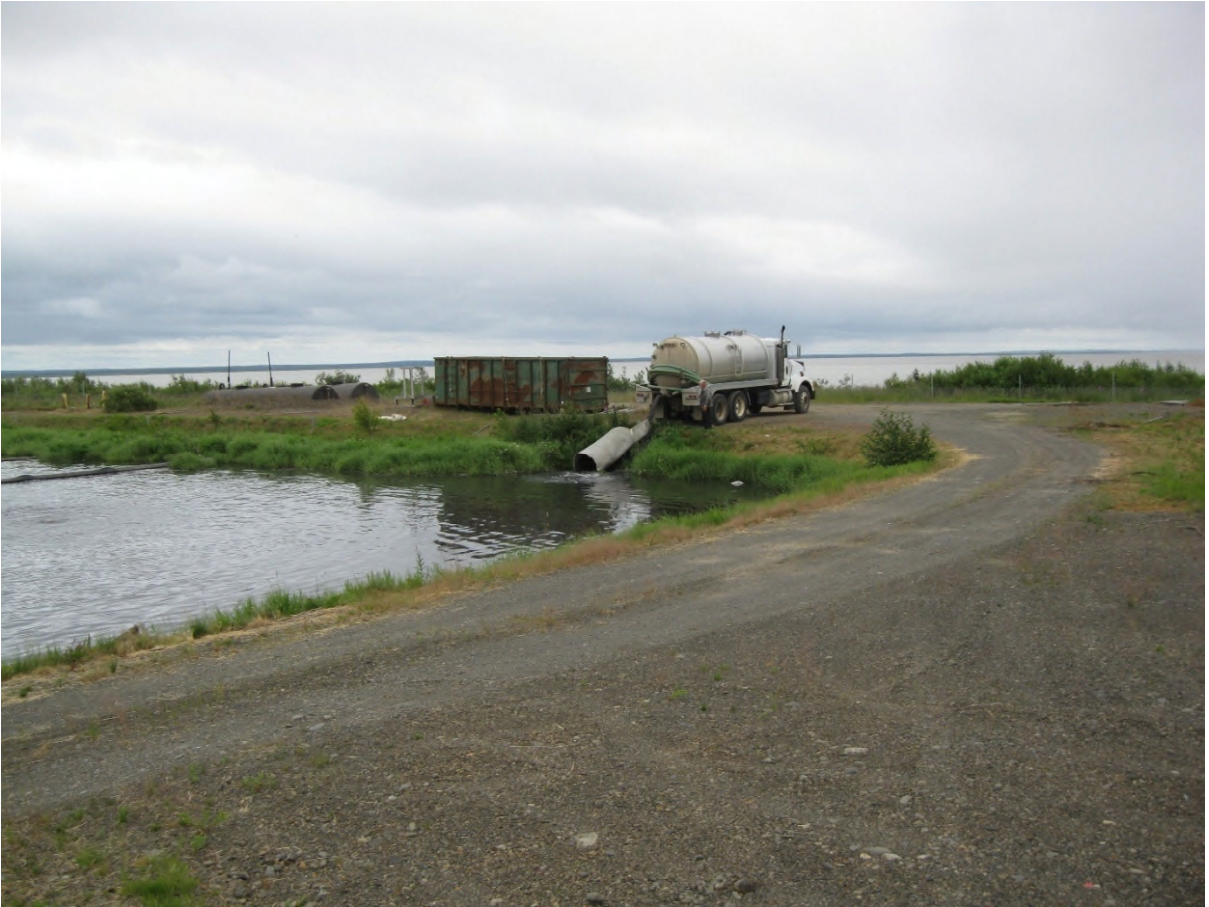
PHOTOGRAPH 1 – PUMPER TRUCK DUMPING AT EXISTING LAGOON SE CORNER CELL #1 (7/12/19)
